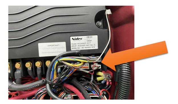
**Step Four.** If the light is flashing the board has an error it will blink in a series of fast flashes and then slow flashes. Count the flashes and see the table below to get your hex code. See document Kinetec error codes.pdf to find what is wrong with your machine. Example 4 fast and 10 slow would be code 4A.
