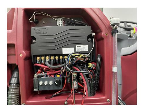
**Step Three.** Find the red light in the bottom right of the controller.
